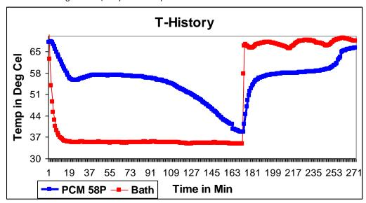
A 30g sample is taken in a test tube in molten condition and placed in a temperature controlled bath. A temperature sensor is placed in the test tube and bath to record the temperatures using a data logger. The bath is maintained at around 35  $^{\circ}$ C during the freezing cycle and at 69  $^{\circ}$ C (maximum) during the melting cycle.
